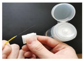
5) Cut the fiber with a fiber optical cleaver.
