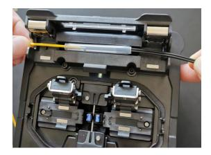
9. Take out the ready fiber and place it to the cooling tray waiting the fiber tube to cool down, then the whole process finished.
