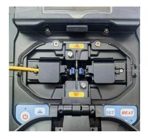
7. Move the heat shrinking tube to the splicing part gently.
