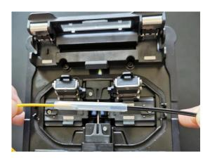
8. Put the fiber to the heating tube, and it will automatically heat.
